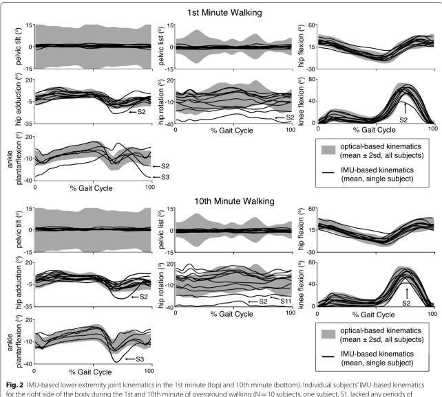
for the right side of the body during the 1st and 10th minute of overground walking (N = 10 subjects, one subject, S1, lacked any periods of straight-walking and was omitted from this plot). Mean  $\pm$  two standard deviations (sd) for optical-based kinematics is shown as a grey shaded band and individual subject means for IMU-based kinematics are shown as black lines
