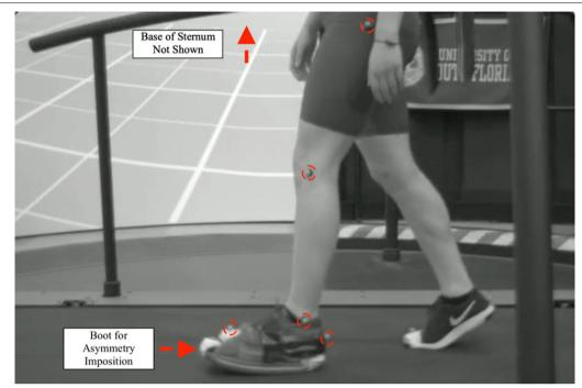
Fig. 1 Marker setup for data collection. Right side has same placement, but not shown in this picture
